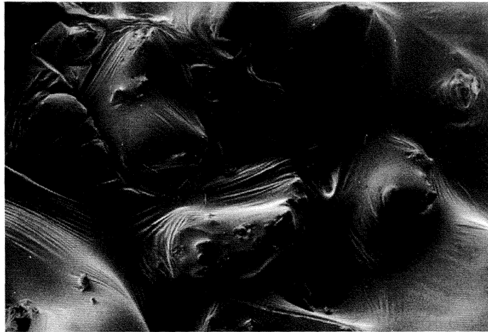
Fig. 6: Influence of application technique on film production. Bituplant was atomized, film is coating the surface of the sand grains and the material hardly penetrates the soil surface (electron microscope, enlarged 500 times)
