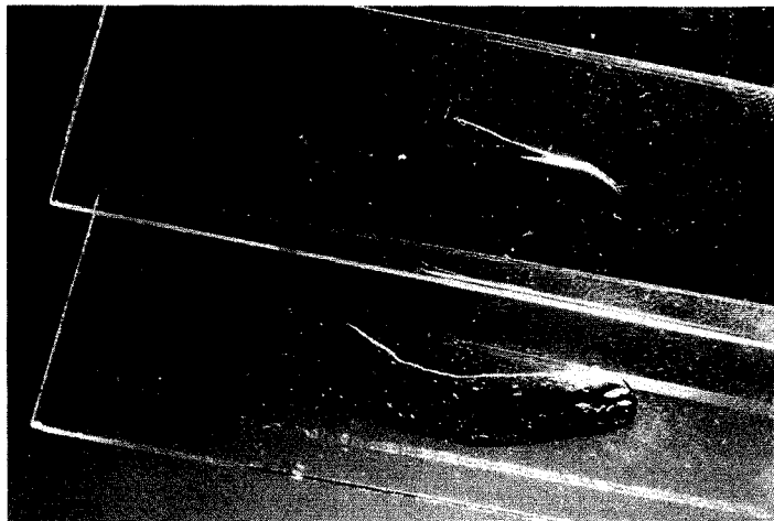
Fig. 1: Spreadproduct for investigating soil stabilizers and evaporation inhibitors concerning their spraying capability. Above: fine bituminous emulsion, easily sprayed. Down: granular emulsion, hardly sprayed
