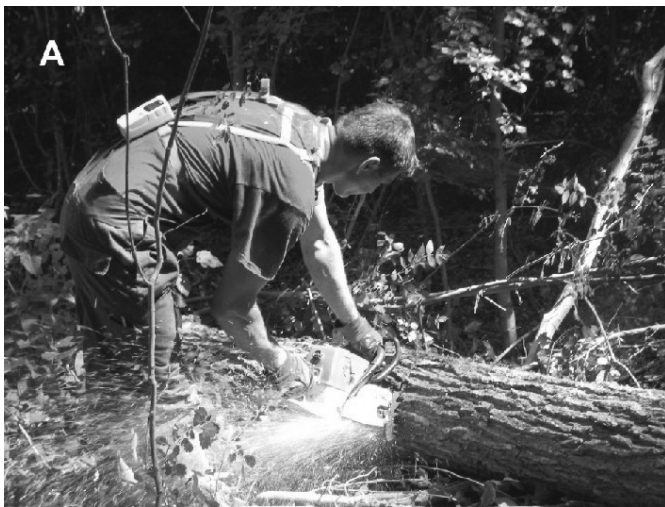
Figure 1: Cutters with attached dust samples A – Processing of fuelwood in summer thinning B – Final cut in winter
