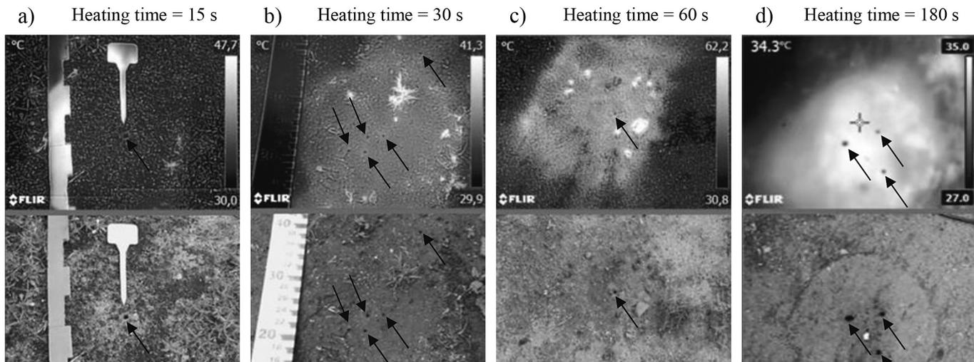
Figure 2: Thermograms (top) and photographs (bottom) of four soil surface conditions recorded *in situ*, in the field. The location of the images, in Recife, is not always the same. The black arrows point out the location of the macropores, created by ants, at the soil surface. The macropores, with a few millimetres are visible at naked eye. The big circles perceptible in the images were created by the plastic container hold against the soil surface (see Figure 1)
