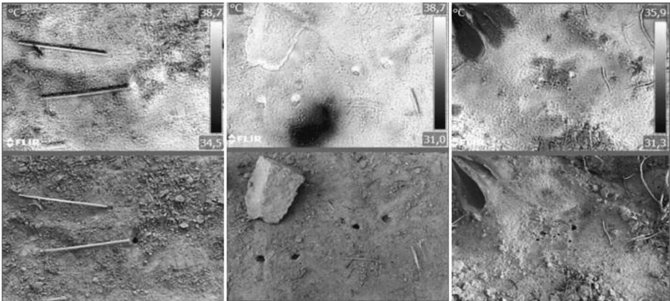
Figure 3: Thermograms (top) and photographs (bottom) for three soil surface conditions tested in the field, without providing any artificial heating of the soil surface
