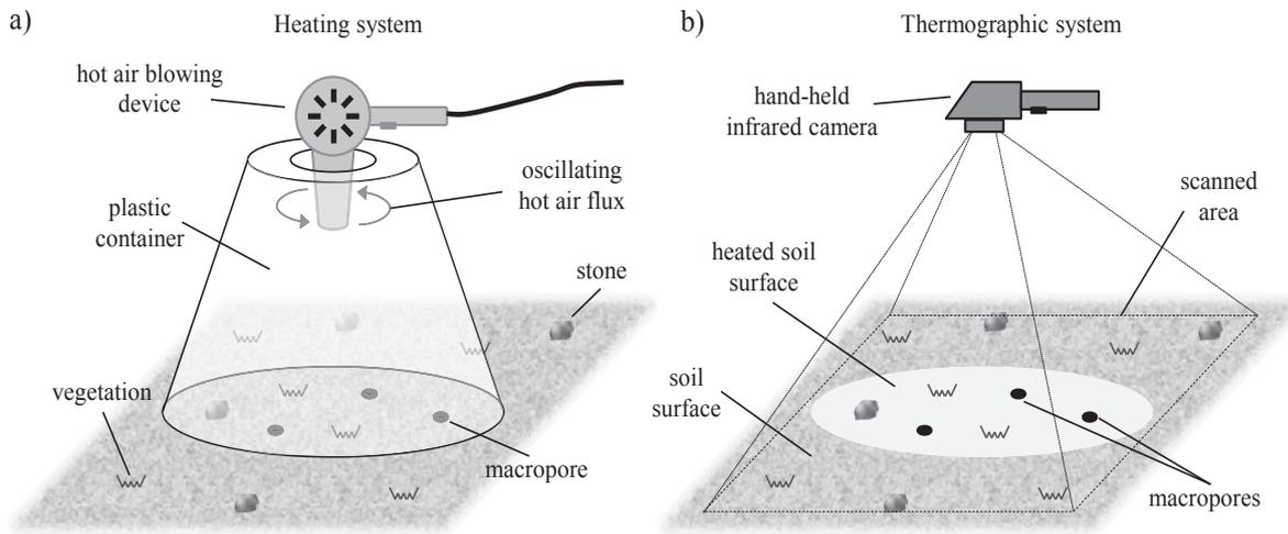
Figure 1: Two phase technique: a) Soil surface heating with hot air blowing system; and b) Thermal scanning of soil surface
